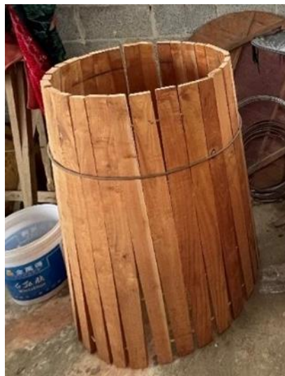
Figure 29 Use the auxiliary bracket to fix the plank
