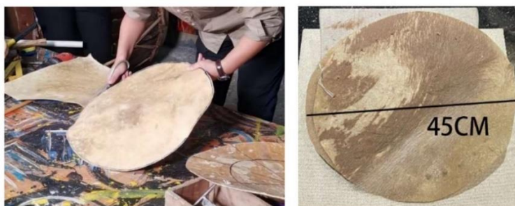
Figure 24 Cutting of cowhide
