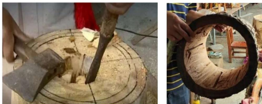
Figure 21 Cutting through shaded wood with a chisel.
