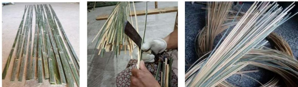
Figure 26 The making of ZhuMie
