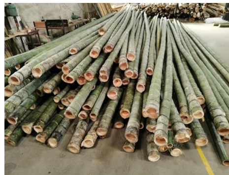
Figure 19 ZhuMie raw material, untreated bamboo
