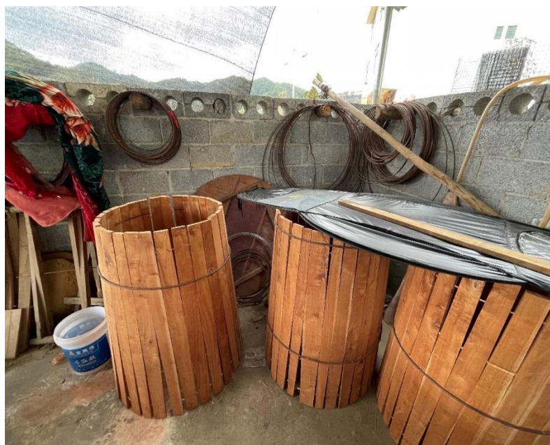
Figure 73 The process of splicing the drum body in the splicing process
