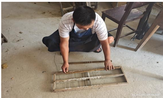
Figure 22 Locate the sound holes by using molds
